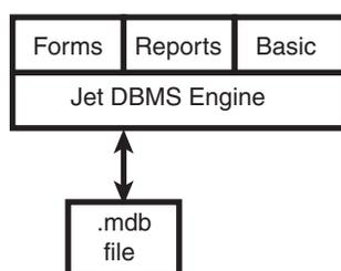
In a single-user Microsoft Access application, the .MDB file and Microsoft Access are located on the same system. In a multi-user Microsoft Access application, the .MDB file is placed on a file server and shared. Each client runs a copy of Microsoft Access and Microsoft Jet database engine. In this configuration, Microsoft Jet database engine must move a large amount of data across the network, including whole tables, to complete its query processing.
