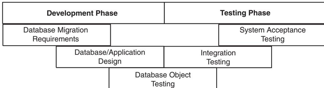
There are several types of tests that you use during the migration process. During the testing stage, you go through several cycles of testing to enhance the quality of the database. The test cases you use should make sure that any issues encountered in a previous version of the Oracle database are not introduced again.
